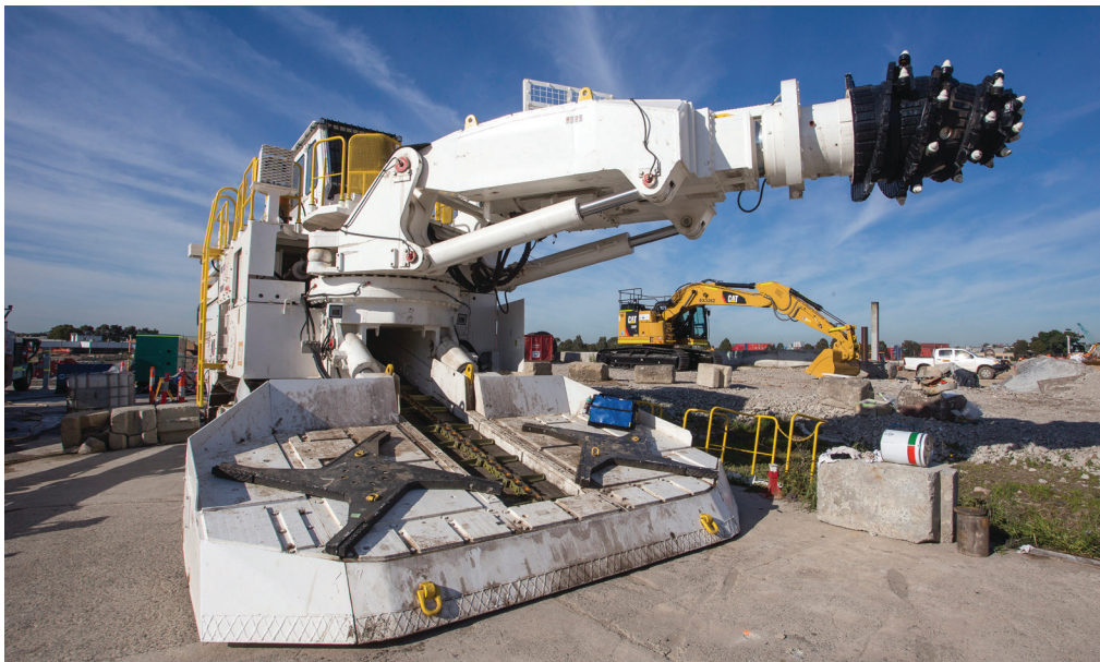
Roadheader tunnelling machine
