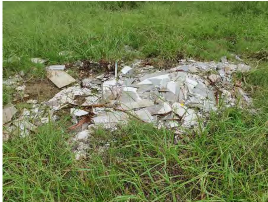
Photograph 17 – Southern Precast Site – Fly tipped fibrous boarding potential asbestos containing material (onsite)
