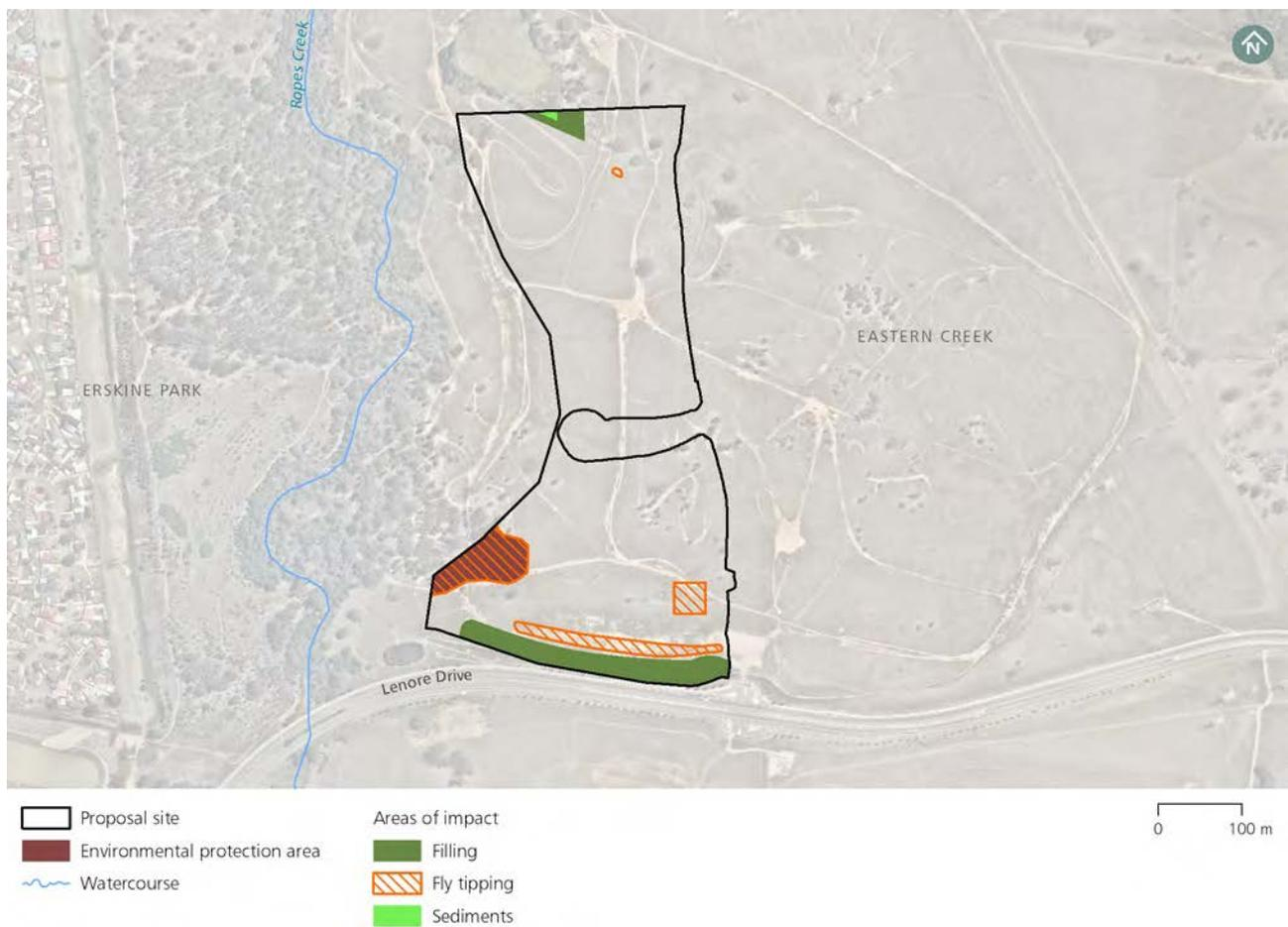
Figure 8-1 Moderate potential contamination impact areas
