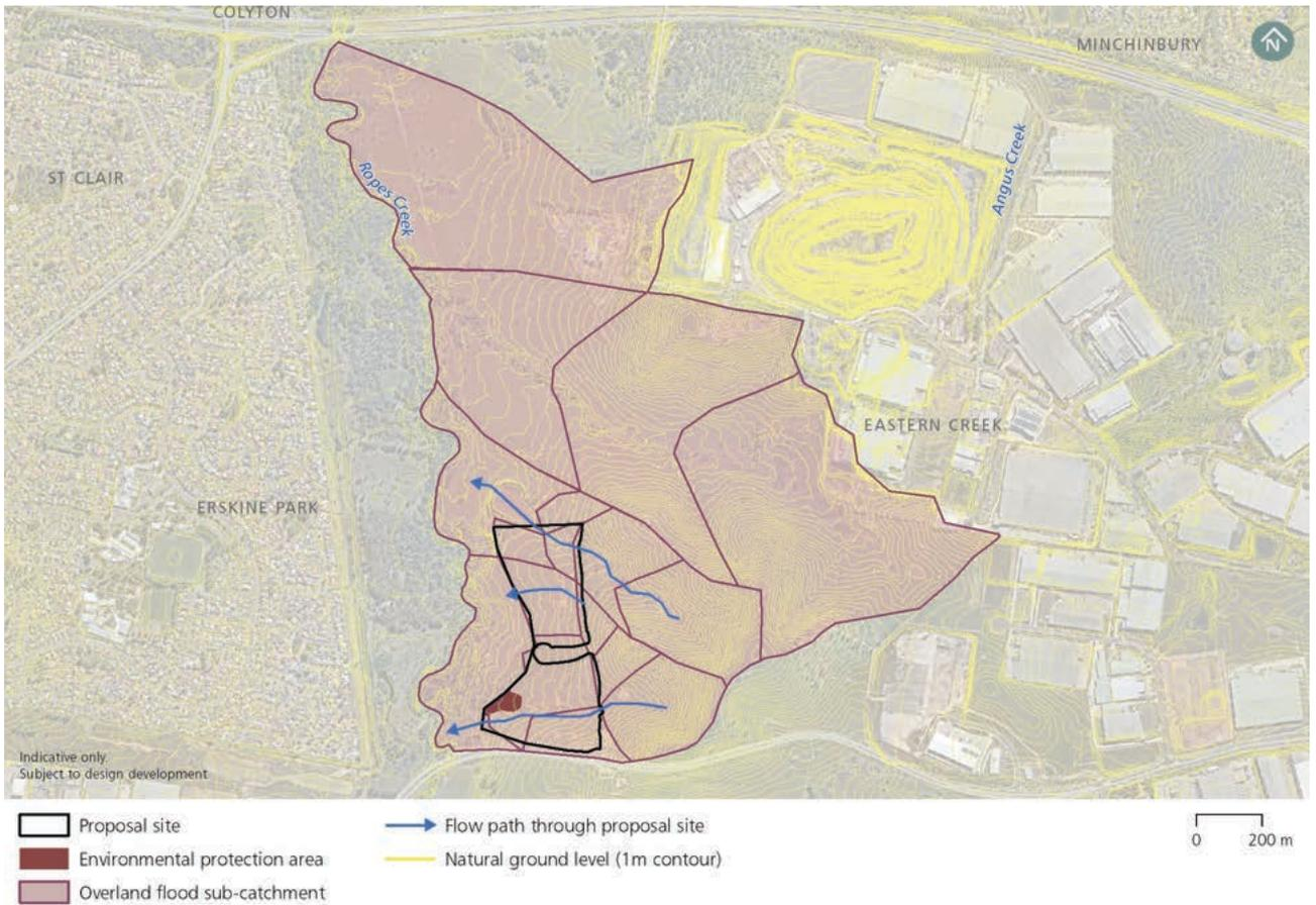
Figure 8-19: Terrain and hydrologic sub-catchments at the proposal site and surrounds
