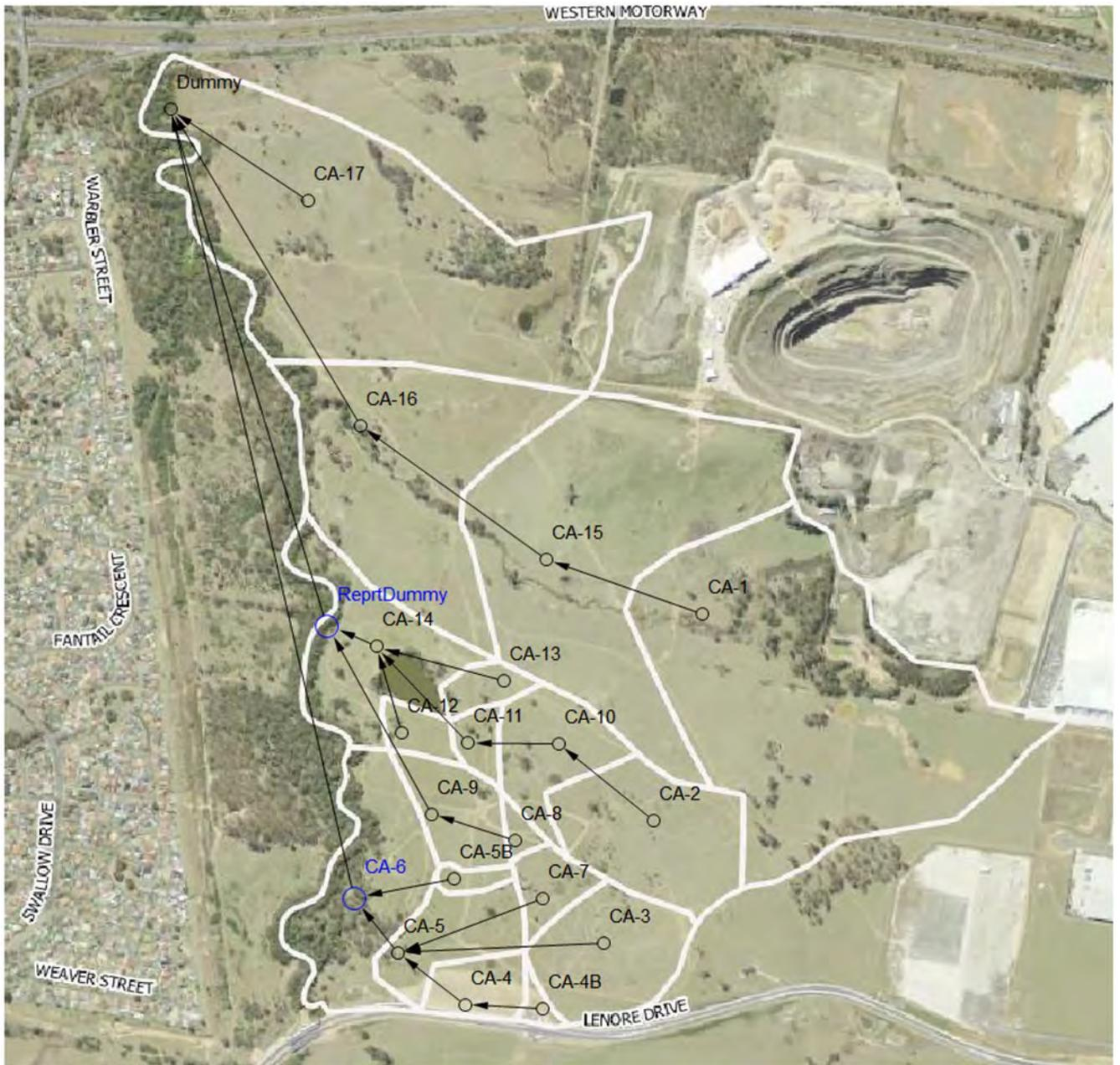
Figure A-2: XP-RAFTS layout – Existing case
