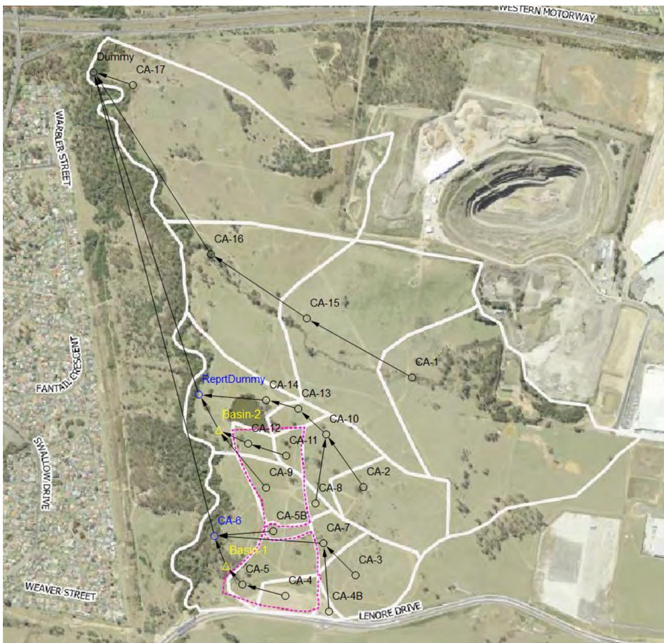
Figure A-6: XP-RAFTS layout – Mitigation case (construction and operational)
