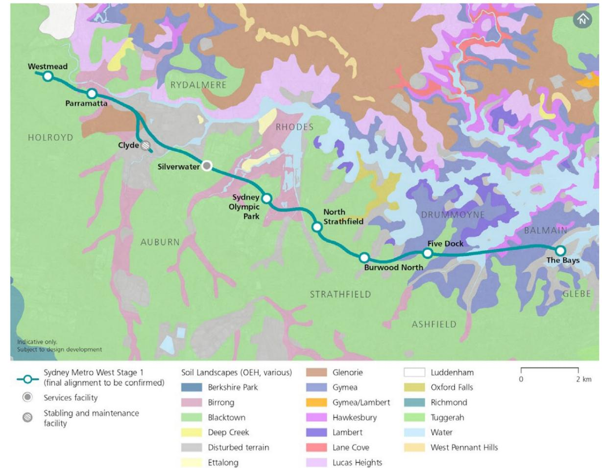
Figure 19-1: Soil units underlying Stage 1
