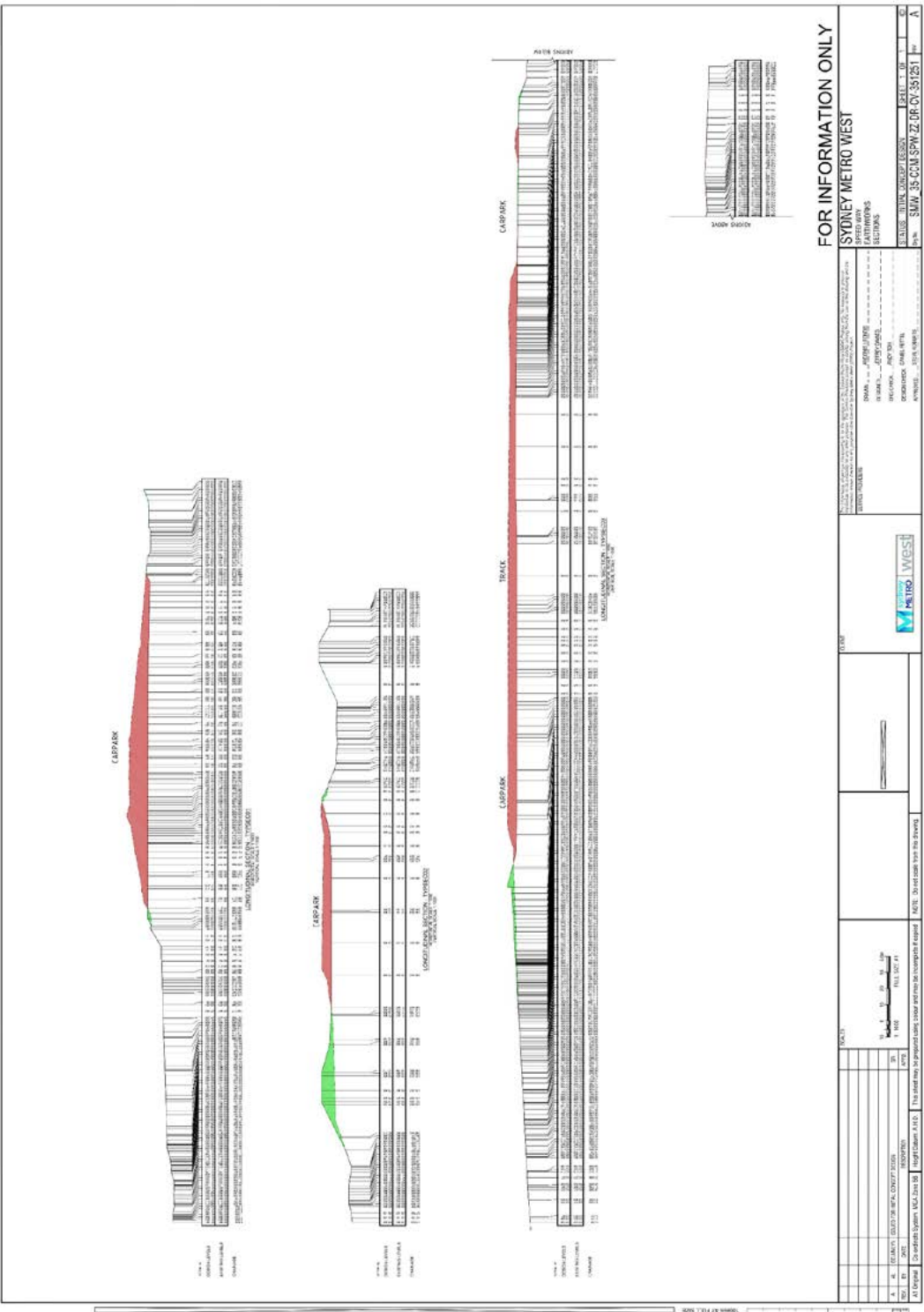
Figure 9 Indicative elevation diagram of cut and fill for project (land reduced indicated in red, land raised indicated in green) (15 April 2020 concept design)
