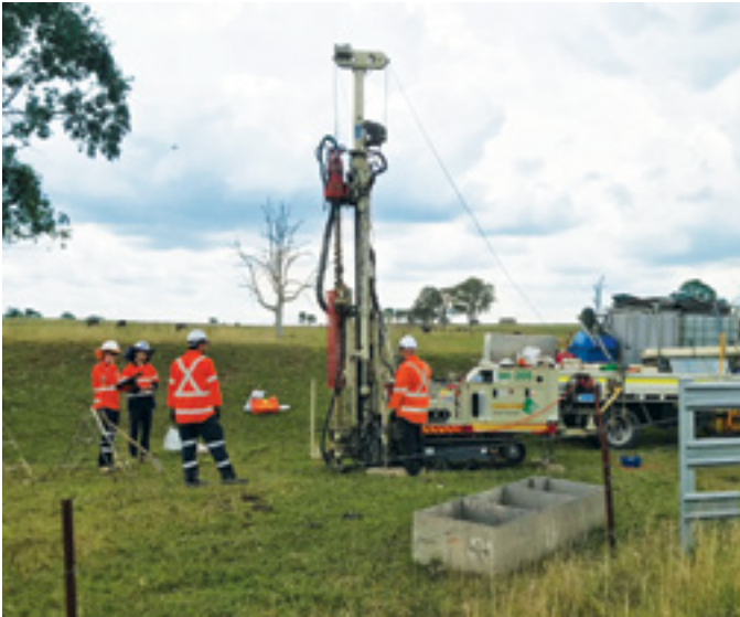
Drilling boreholes to collect samples along the M12 Motorway corridor
