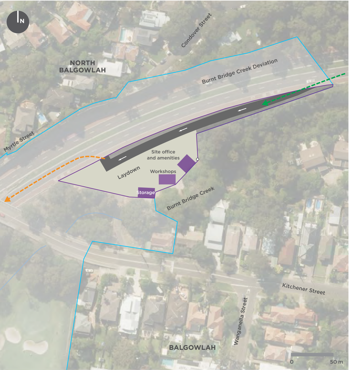
Kitchener Street temporary construction support site
