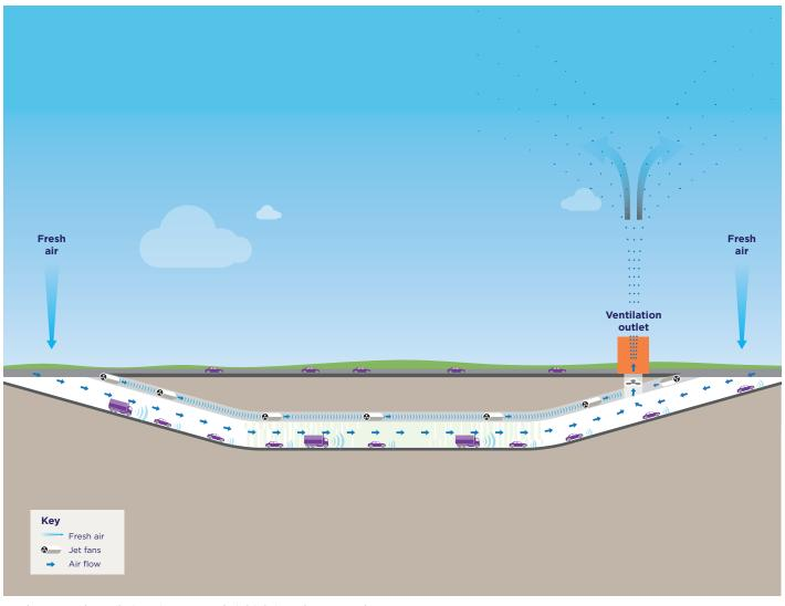
Modern tunnel ventilation ejects tunnel air high into the atmosphere
